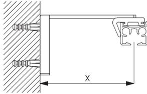
**Smart Fix SG 11200 - SG 11205 and bracket SG 3826:**
